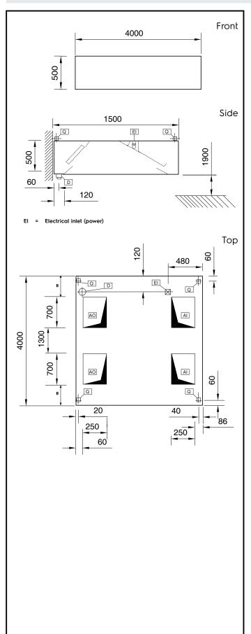
**Electric** Supply voltage: 641264 (STPF1540) 220 V/1N ph/50 Hz **Total Watts:** 0.32 kW Capacity: Supply capacity: 3960 m<sup>3</sup>/h **Key Information:** External dimensions, Width: 4000 mm External dimensions, Depth: 1500 mm 500 mm External dimensions, Height: Net weight: 246 kg Air Emission:
